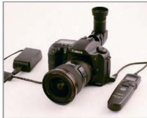
A DSLR equipped with a programmable remote control (intervalometer), an AC adapter, and an angle finder
